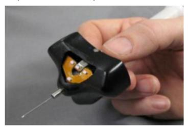
Figure 1. The MICRON. A hand-held robotic manipulator.
