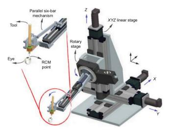
Figure 3. The Steady-Hand Eye Robot (SHER) (RCM, Remote center of motion). Roizenblatt M, Edwards TL, Gehlbach PL. Robot-assisted vitreoretinal surgery: current perspectives. Robot Surg. 2018;5:1-11.
