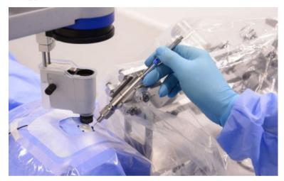
**Figure 2.** The intraocular robotic system of the Catholic University of Leuven. Gijbels A, Smits J, Schoevaerdts L, et al. In-human robot-assisted retinal vein cannulation, a world first. Ann Biomed Eng. 2018;46:1676-1685.
