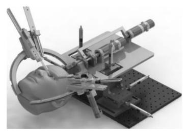
**Figure 7.** Intraocular robotic interventional surgical system (IRISS). Gerber MJ, Pettenkofer M, Hubschman JP. Advanced robotic surgical systems in ophthalmology. Eye (Lond). 2020;34:1554-62.
